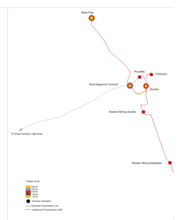
The diagram above shows the 220kV transmission line supplying the Eastern Goldfields region from the East Country Load Area (Merredin Terminal).
