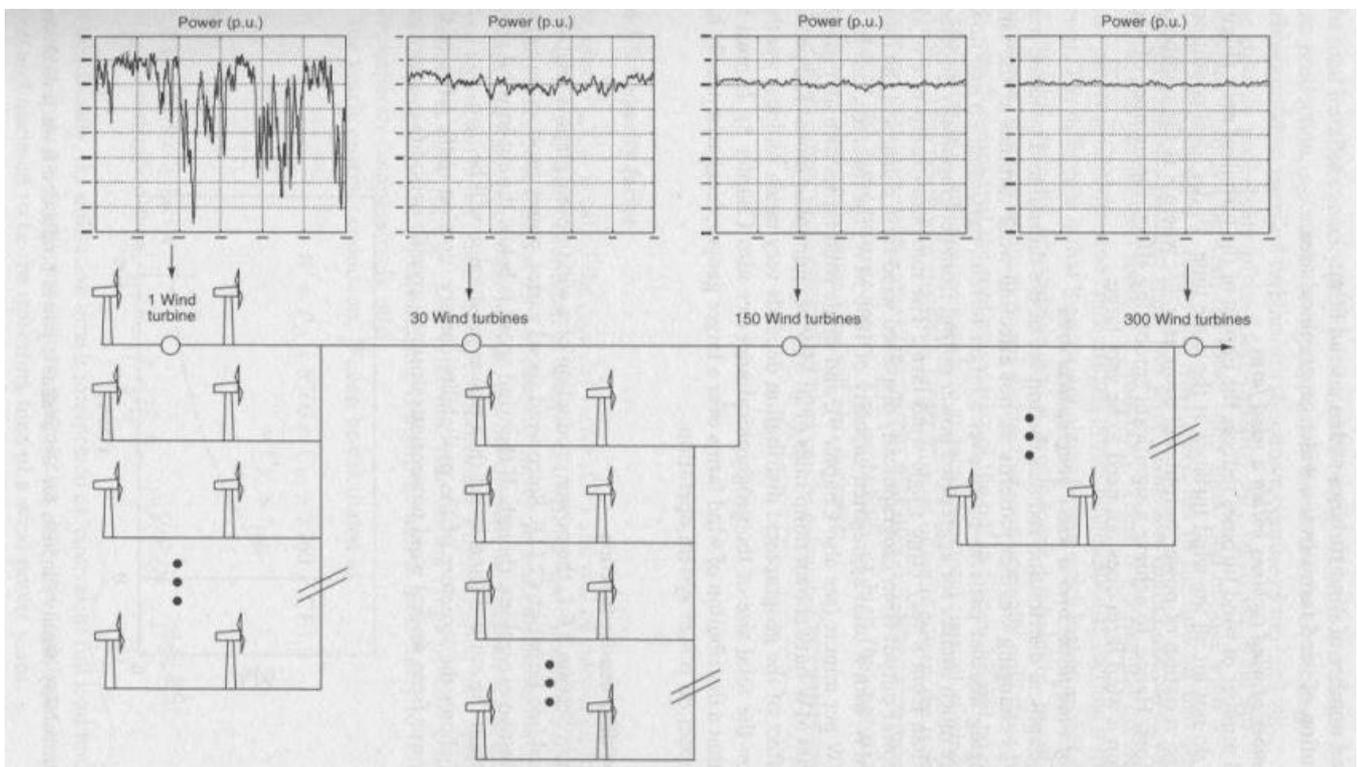
**Figure 3.7** Impact of geographical distribution and additional wind turbines on aggregated power production. Time scale on graphics: seconds. Based on simulations by Pedro Rosas (Reproduced from P. Rosas, 2003, *Dynamic Influences of Wind Power on the Power System* (PLD thesis, Ørsted Institute and Technical University of Denmark), by permission of Pedro Rosas.)
