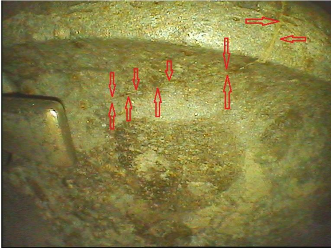
Figure 0.1: Typical crack discovered with borescope on the CS7/2 first stage blade
