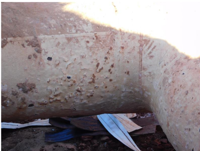
Unit discharge pipework failed coating system
