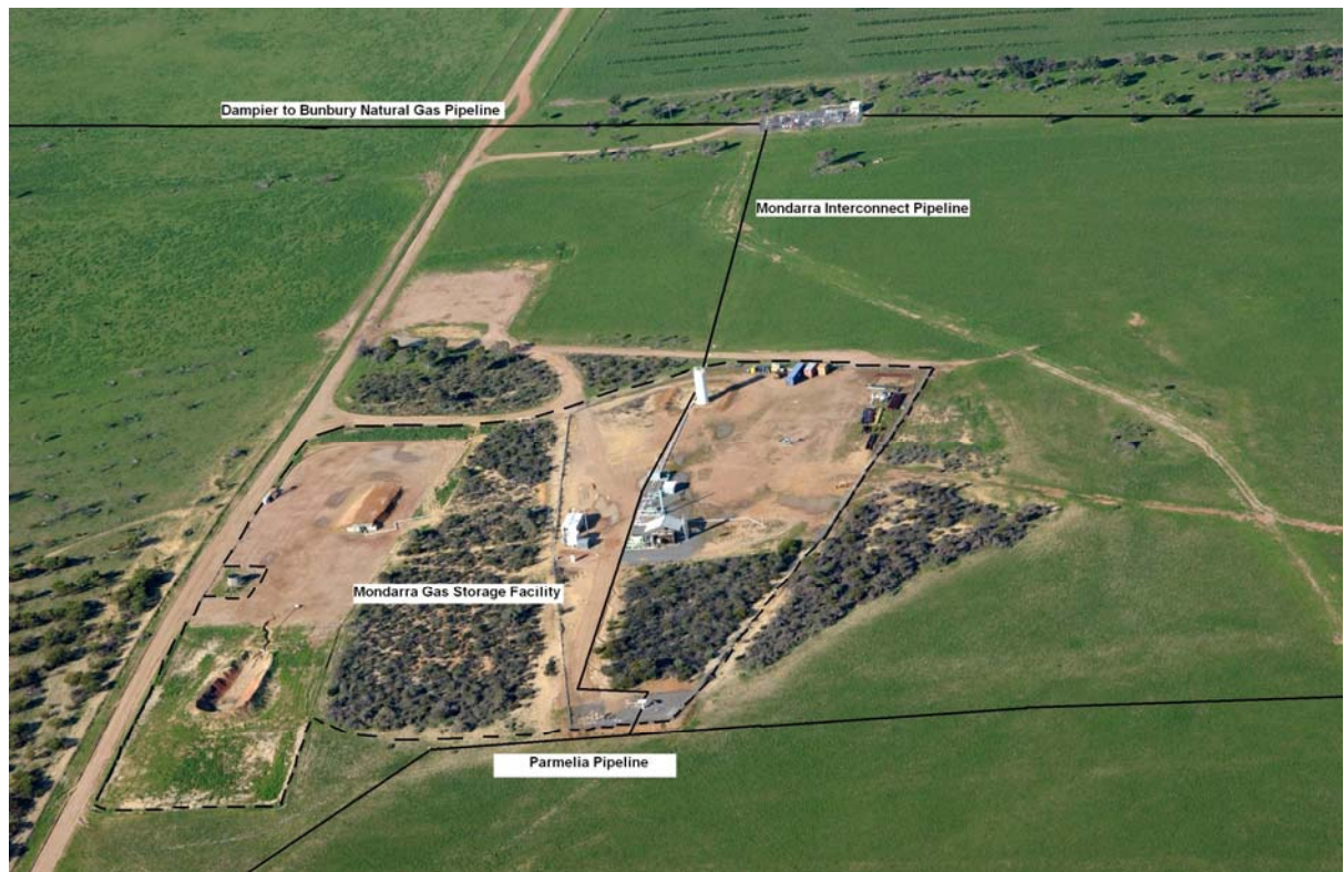
Figure A3-1: Mondarra Gas Storage Facility: Layout and Pipeline Interconnections and Locations
