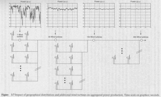
Figure 3.7 Impact of geographical distribution and additional wind turbines on aggregated power production. Time scale on graphics: seconds. Based on simulations by Pedro Rosas (Reproduced from P. Rosas, 2003, *Dynamic Influences of Wind Power on the Power System* (PLD thesis, Ørsted Institute and Technical University of Denmark), by permission of Pedro Rosas.)
