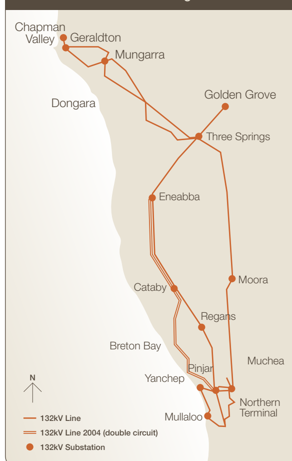
Figure 1: Overview of transmission network in the Mid-West region
