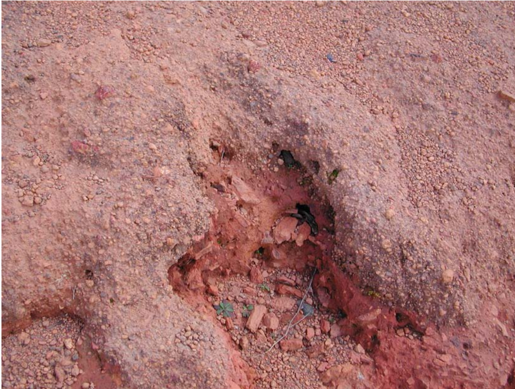
Plate 4.3 : Honeycomb feature below FSL along the upstream reservoir rim on the right abutment
