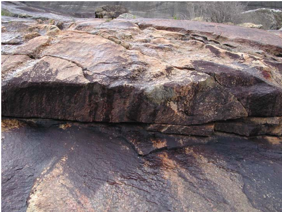
Plate 4.9 Disadvantageous joint orientation in foundation rock
