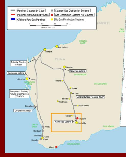
Owner: Southern Cross Pipelines Australia Pty Ltd Commissioned: 1996 Length: 44 km Diameter: 219 mm Capacity: 15 TJ/d Throughput: 12 TJ/d Extension of time to submit an Access Arrangement granted to July 2004
