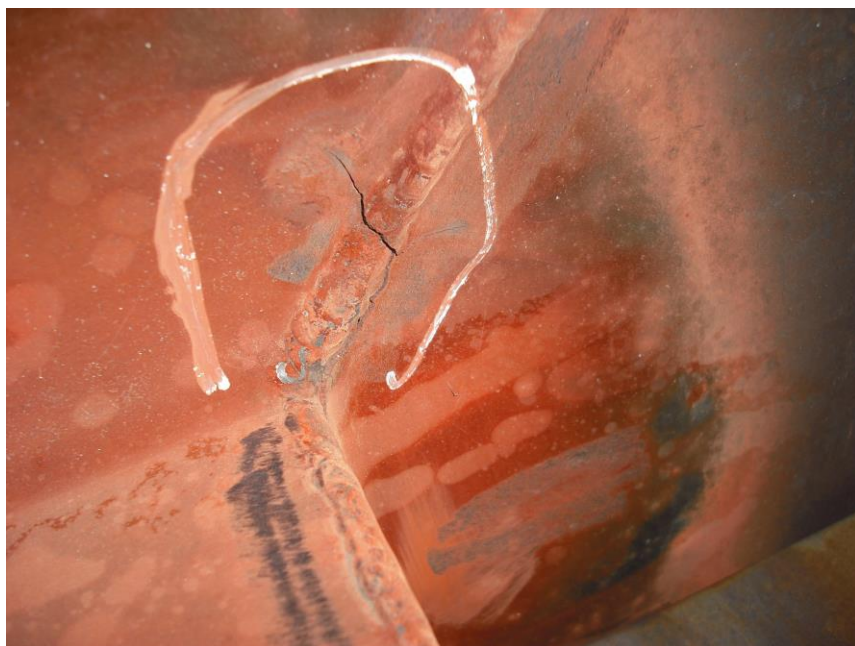
Figure 3: Exhaust bellows cracking on CS5 U2 (August 2019)
