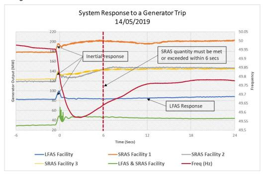
The red solid line indicates system frequency. The blue line indicates a Facility providing LFAS only. The green line indicates a Facility providing both LFAS and SRAS. The red dotted line indicates the time (6 secs) within which SRAS quantity must be met or exceeded. The remaining lines indicate Facilities providing SRAS only.
