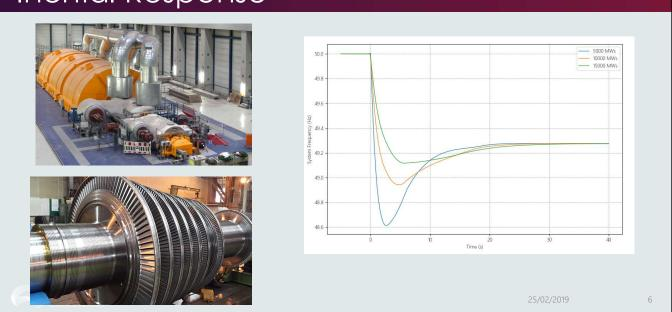
Inertia defines how quickly the frequency changes immediately after a contingency.
