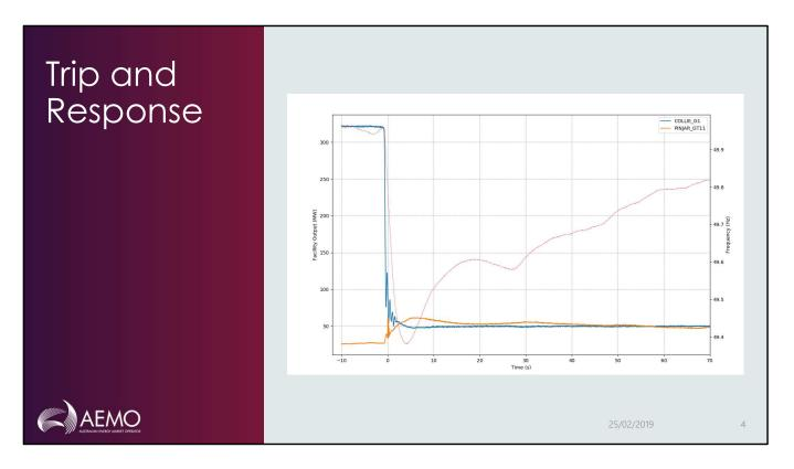
Pinjar "only" replaced 35 of ~300 MW; other machines in the fleet made up the rest.
