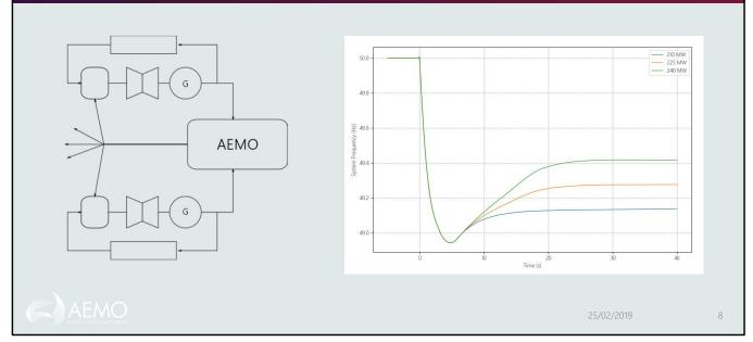
SFR is characterised by system-wide control, typically through coordinated changes to the setpoints of multiple facilities (e.g. via an Automatic Generation Control system). Its reaction time is limited to the refresh rate of the control system (on the order of 4 - 20s) and draws on rate-limited but more stable and sustainable machine processes.
