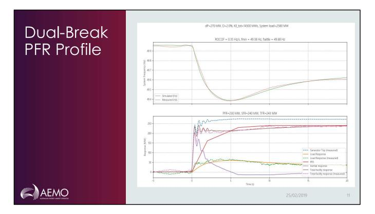
Through experimentation, a robust fit was found using a "dual break" PFR profile, characterised by an initial fast ramp from 0 - 2s, followed by a slower ramp to 6s. The best-fit profile is shown in Figure 8 (bottom), along with various other signals of interest. In these plots, dashed lines are measured values, while solid lines show simulation output.
