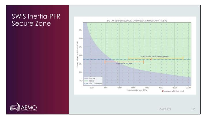
With the calibrated model, the dual-break PFR profile defines the security limit which aggregate machine response must exceed to ensure a minimum nadir frequency.
