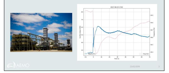
Pre-fault ~25 MW. Unit is synchronised purely for spinning reserve.
