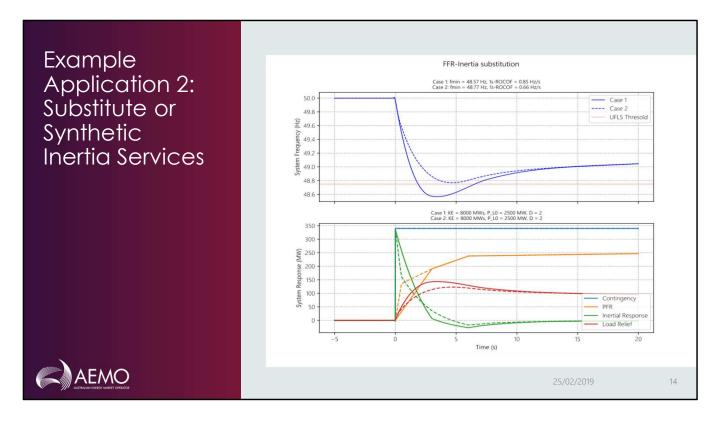
The terms "fast frequency response" (FFR) and "synthetic inertia" both refer to the concept of technology with a fast-enough contingency response to limit system ROCOF, and thereby serve as a substitute for system inertia. While the 2s breakpoint was chosen to match the observed capability of facilities currently active in the WEM, the aggregate model provides a straight-forward means to investigate and quantify the impact of introducing faster contingency responses to the overall mix.
