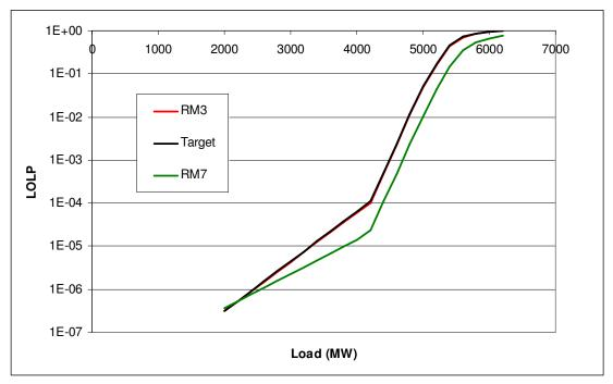
Figure 6-3 LOLP versus the load for scheduled generation
