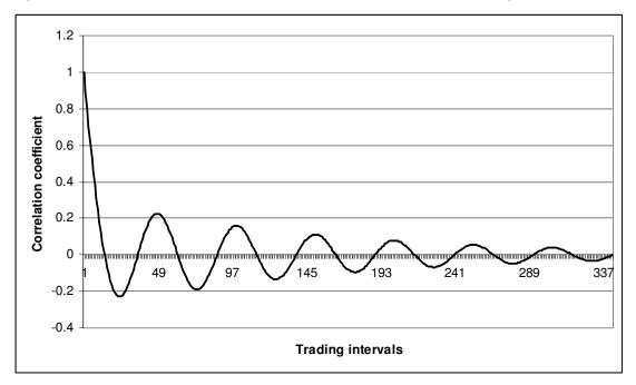
Figure 6-8 Example of correlation of wind farm output between trading intervals
