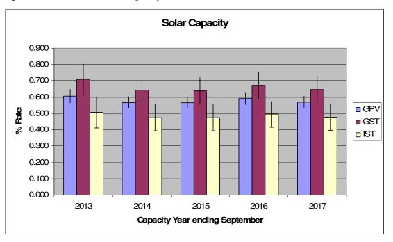
Figure 6-22 Assessed LOLP capacity values for solar resources
