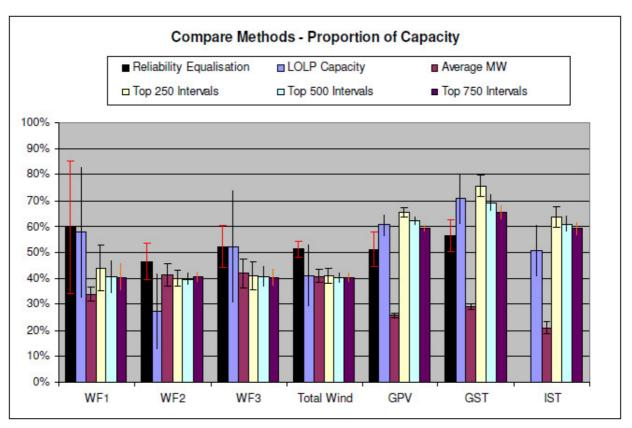
WFx = actual Wind Farm x (not identified due to data confidentiality) GPV = simulated Geraldton Photo-Voltaic solar farm GST = simulated Geraldton Solar Thermal plant IST = simulated Inland Solar Thermal plant
