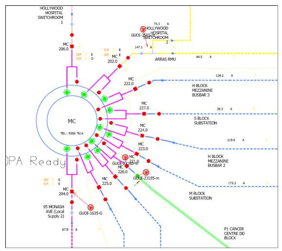
Figure 14: Medical Centre distribution feeder circuits
