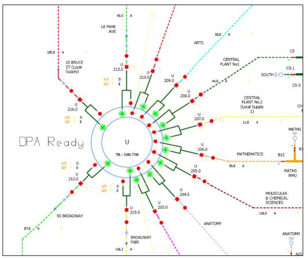
Figure 15: University distribution feeder circuits
