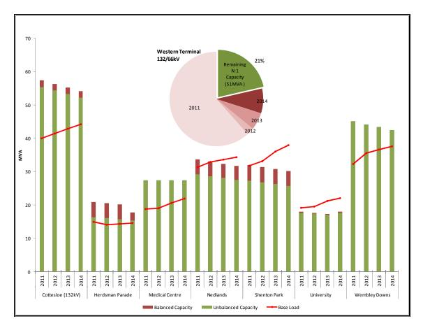
Figure 5: Western Terminal load area substation capacity summary (2011-2014)
