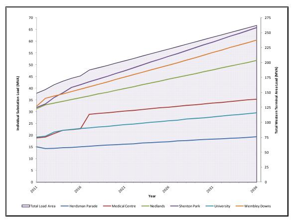
Figure 4: 2011-2036 load forecast (10% PoE) for the Western Terminal load area
