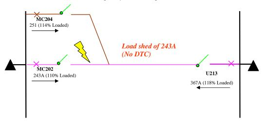
Figure 10: Fault during summer 2014/15 peak loading (MC202 off-load scenario)
