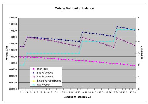
Figure 17: Load unbalance vs. Voltage (66kV)
