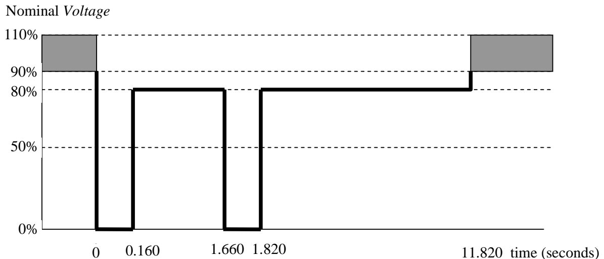
Figure 3.6 - Off nominal voltage operation capability requirement for generating units during auto-reclose operation
