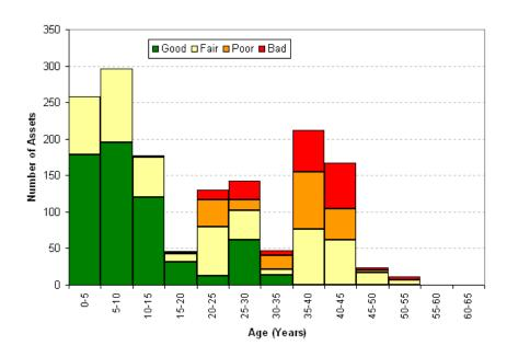
Figure 7.25: Outdoor Circuit breaker condition profile
