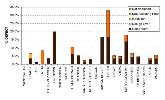
Figure 7.30: Disconnectors failure mode and manufacturer
