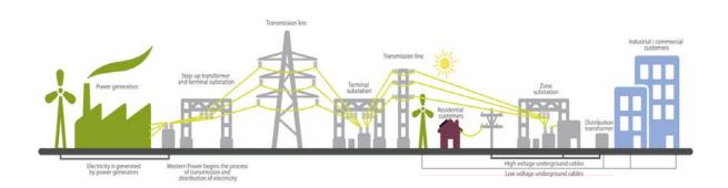
Figure 1.3: How Western Power transports electricity (green is transmission and red is distribution)
