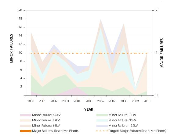
Figure 7.43: Reactive plant failure comparison in the last 10 years
