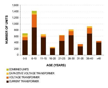
Figure 7.36: Age Profile of Instrument Transformers
