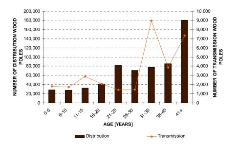
Figure 7.17: Age profile of distribution and transmission wood poles
