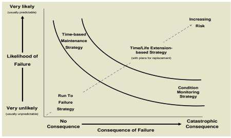
Figure 4.7: Potential strategies responding to likelihood of failure and consequence of failure
