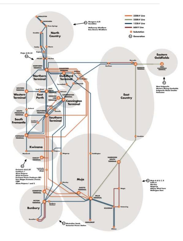
Figure 6.1: Load areas in the Western Power's electricity network
