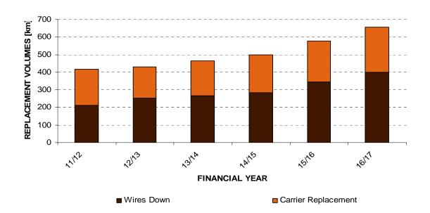
Figure 7.11: Planned volumes for replacement under Wires Down and Carrier Replacement programs
