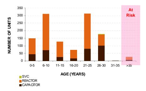
Figure 7.41: Transmission reactive plant age profile
