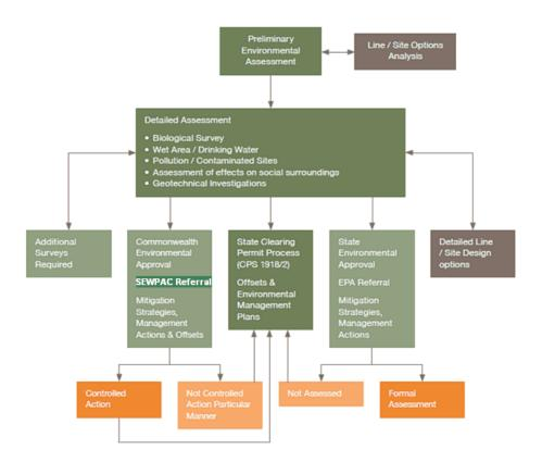
Figure 6.2: Environmental approval process
