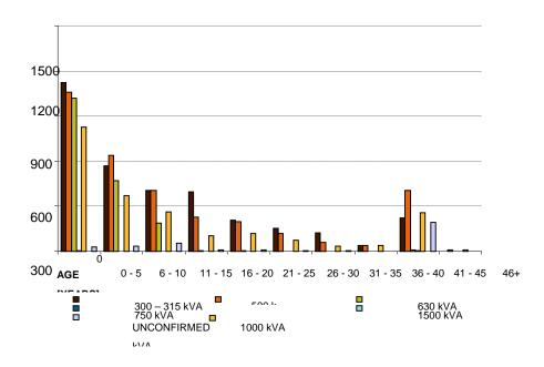
Figure 7.55: Ground mounted distribution transformer ≥ 300 kVA age profile
