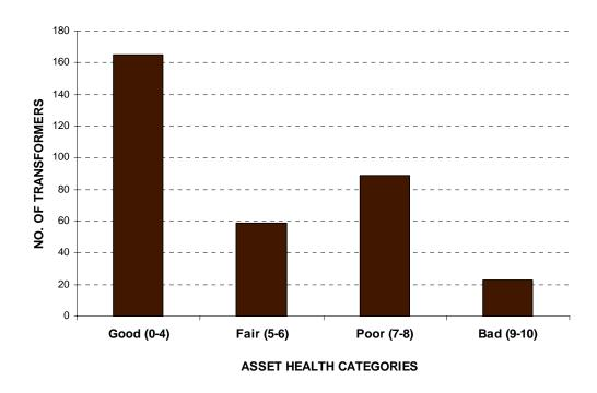
Figure 7.5: Power transformer condition rating
