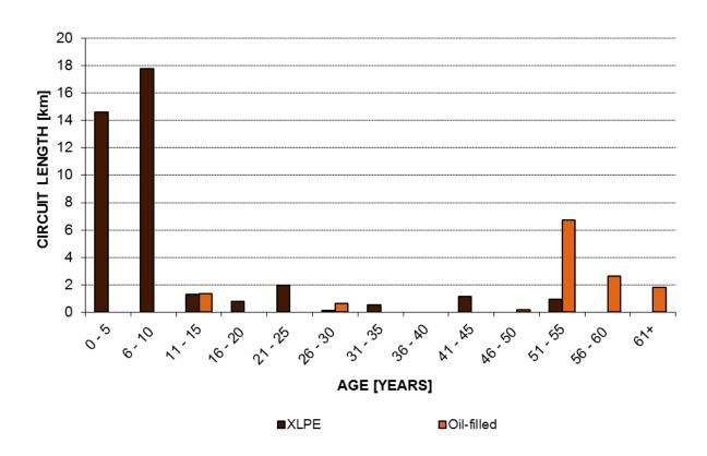
Figure 7.14: Transmission cables age profile
