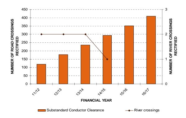
Figure 7.13: Planned volumes of road and river crossings to be rectified under the Substandard Conductor Clearance program and Distribution River Crossing program
