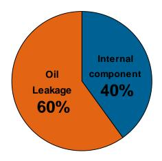
Figure 7.21: Circuit breaker failure modes
