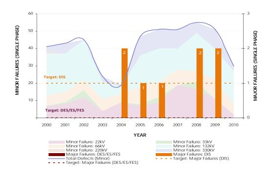
Figure 7.31: Disconnectors defects and major failures history
