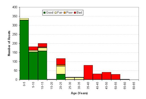
Figure 7.24: Indoor Circuit breaker condition profile
