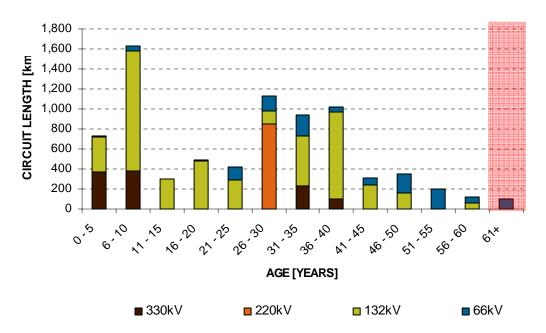
Figure 7.9: Age profile of overall transmission overhead conductors
