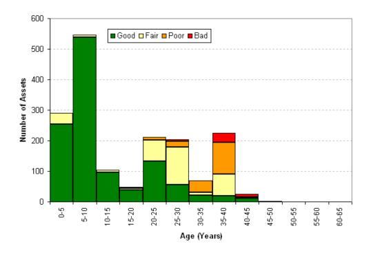
Figure 7.39: Condition Profile of Voltage, Capacitive Voltage Transformers and Combined Units
