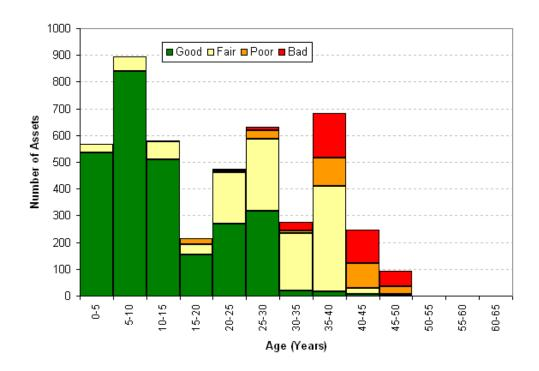
Figure 7.38: Condition Profile of Current Transformers
