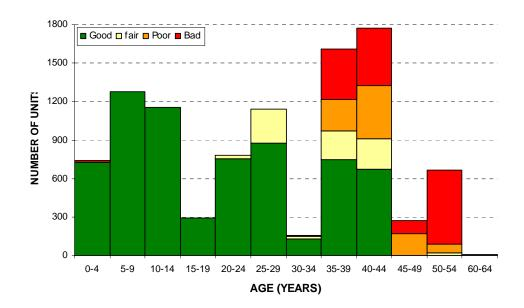
Figure 7.33: Disconnectors condition profile
