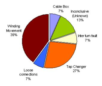
Figure 7.4: Major transformer failures (since 1997)
