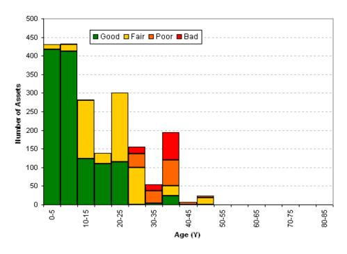
Figure 7.62: Transmission surge arrester condition profile
