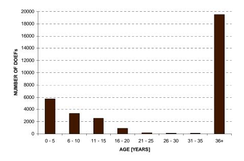
Figure 7.50: Drop out expulsion fuse age profile
