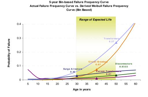
Figure 4.8: Time to failure probability distribution curve
