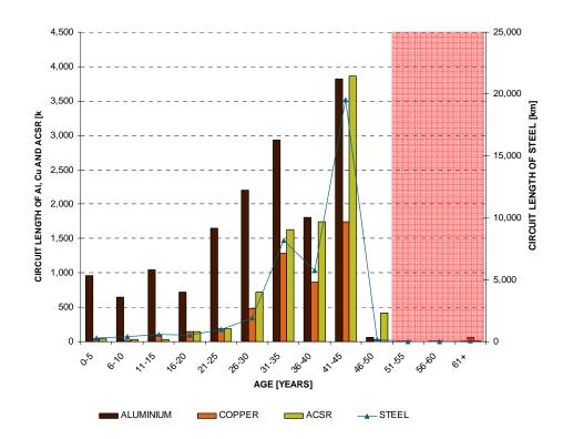
Figure 7.10: Age profile of distribution overhead conductors by type
