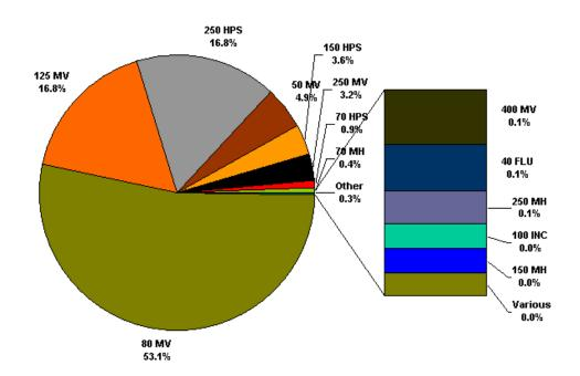
Figure 7.57 Streetlight types by globe type
