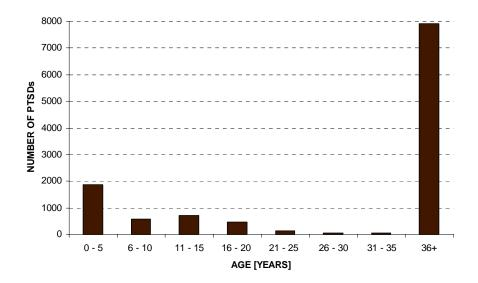
Figure 7.49: Pole Top Switch Disconnector age profile
