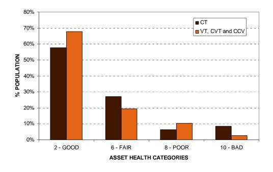
Figure 7.37: Instrument transformer condition rating
