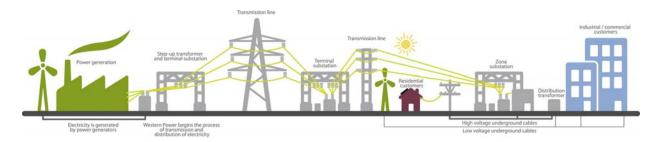
Figure 3.1: How Western Power transports electricity
