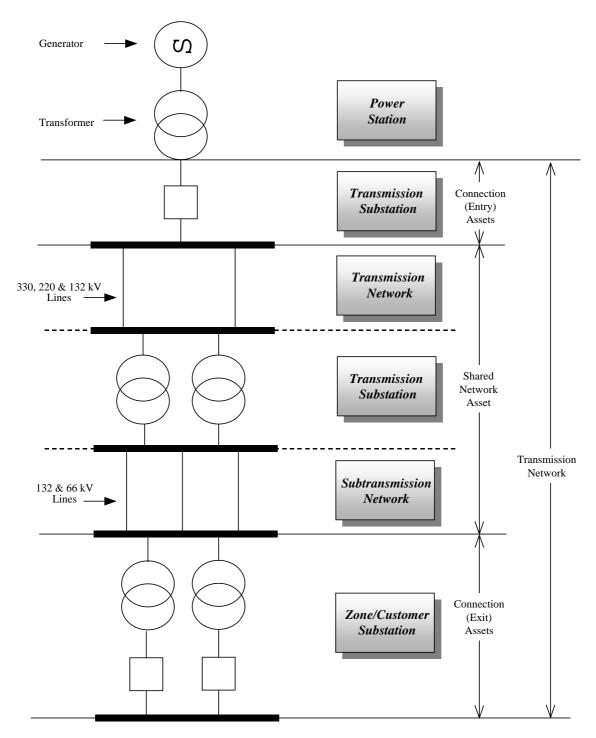
The Western Power transmission network system includes high voltage (330kV, 220 kV, 132kV and 66kV) primary equipment at power stations (excluding low voltage primary equipment and step-up transformers at the generator switchyard), high voltage transmission lines, transmission substations, subtransmission lines and the zone/customer substation equipment at the interface with the distribution business.
