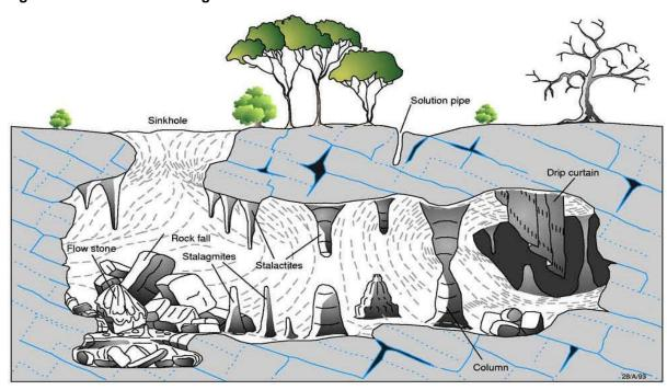
Figure 12.1 Schematic Diagram of a Karst Terrain
